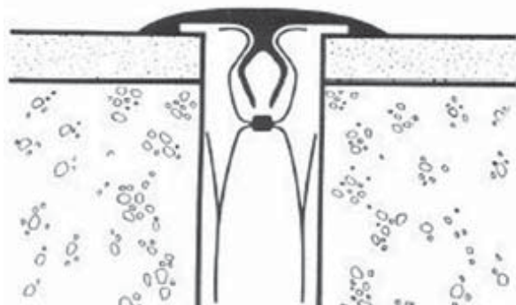
FLOOR - JOINT DETAIL
