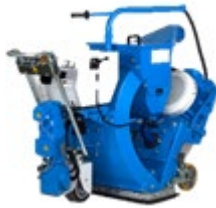
Fig.2: Grit blasting machine
