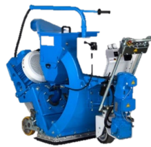
Fig.2: Grit blasting machine
