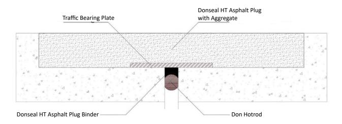
Blockout should be prepared by removing any loose material, latencies and contamination which can affect the adhesion of Donseal HT Asphalt Plug. Blockout should have a minimum depth of around 50 mm and a width of 300 up to 700 mm.
