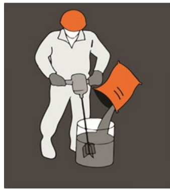
Mixing using drill and mixing paddle
