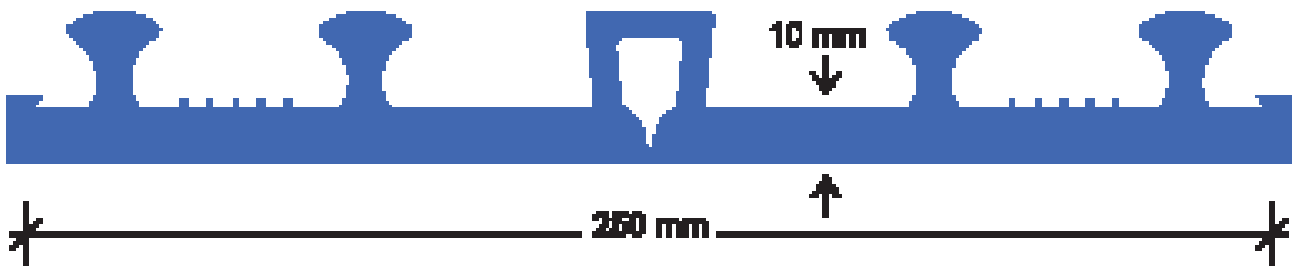
External fix for expansion & construction joints (AB232)
