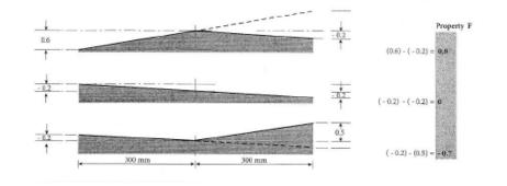
1.4.3 Raised sections should be treated by proper mechanical means like grinding, grit blasting or any other means while all deeper sections should be filled by epoxy mortar like Quickmast 341 to reach a smooth and flat surface as the below figure shows.
